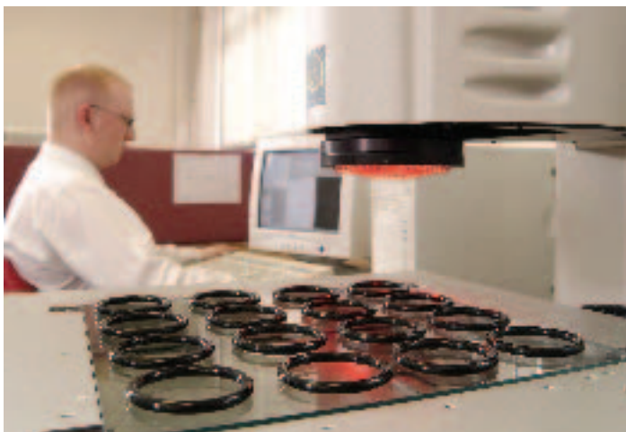
Critical inspection of elastomeric mouldings with state-of-the-art optical measuring system
