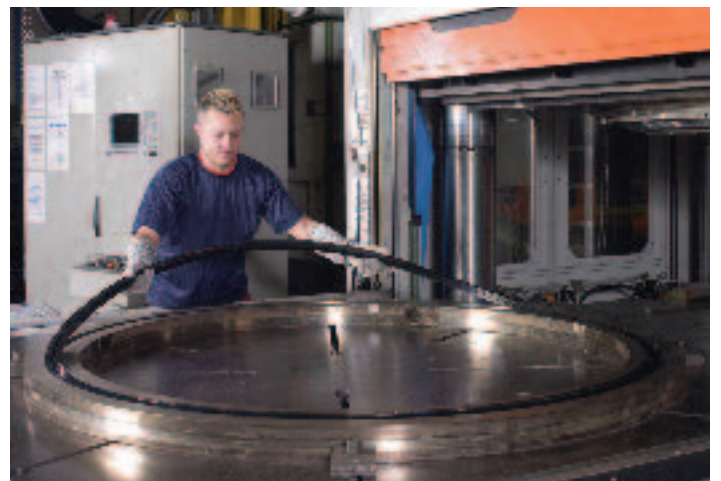
Vacuum moulding at James Walker's Cockermouth plant
